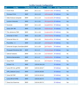
There are two ways to set up a facility ID to connect to the ACLS Logon Server: by its network IP address, or its Host ID generated by the console. The following parameters are required for setting up the console control:
