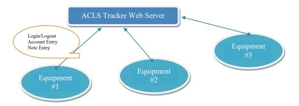
Through the tracker, you can implement a secured access to instrument or equipment by "No Login, No Operation" policy.
