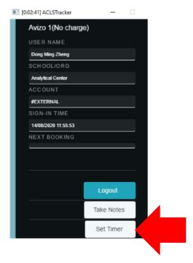
➤ Select the desired hours, and click 'Start Timer' to begin the countdown. Tracker logs out user automatically when countdown ends.
