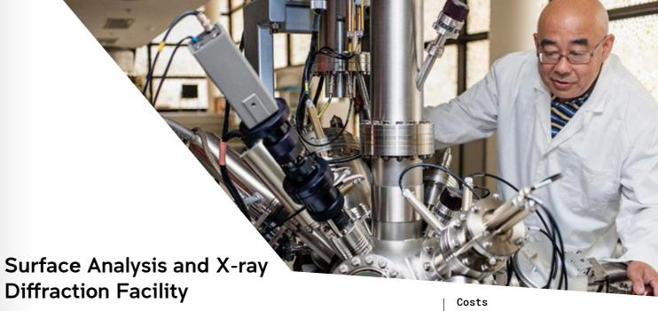
The **Surface Analysis Laboratory** performs chemical analysis of surfaces of solids and powders. Surface chemistry can be measured at the top 5 nm using photoelectron spectroscopy or <1 nm using surface mass spectrometry. Complex samples, such as biological tissues, can be chemically mapped or depth profiled at <1 nm precision.
